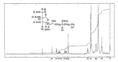
Fig. 2. N.M.R. spectrum of dihydroanhydromyriocin tetraacetate.
